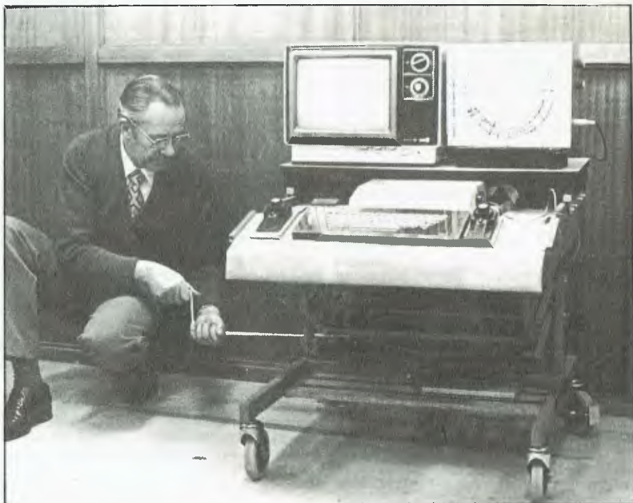
The SCAT (Scanner Apple Touch Keyboard), developed by Centre Industries, the manufacturing division of the NSW Spastic Centre. The SCAT is a self-contained unit incorporating SCAT interface, movable TASA (Touch Activated Switch Array) keyboard and a rotary scanner.
